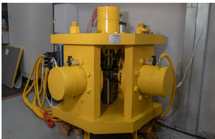
UNIQUE TEST FACILITY FOR FORMATION PRESSURE SIMULATION
